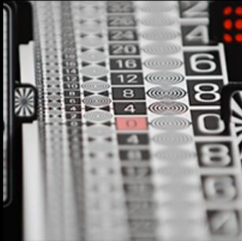
Focus Display Ruler showing back-focus
